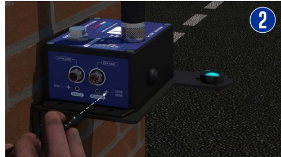
Caption 2: To enable the sensor zeroing function, hold the magnet on "Sensor Zeroing" Label for more than 20s.
