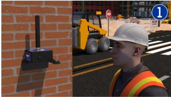
Caption 1: After installing the Alpha-Inc-Kompakt inclinometer, the field operator can check at any moment if the sensor is working properly
