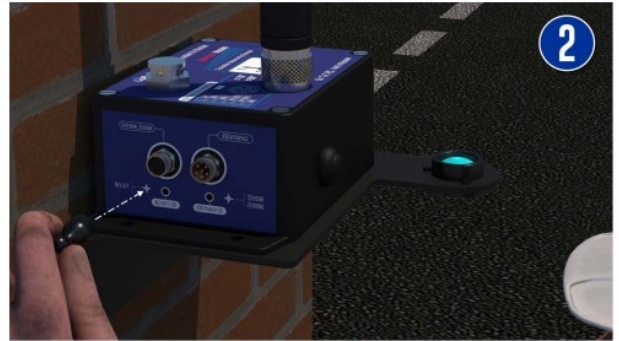
Caption 2: By Holding the magnet on the 'Hello!' label for more than 5s, the sensor wakes-up and transmits to the Lorawan network the data measurement followed by the system diagnostic ( battery status and network quality)
