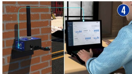
Caption 4: The Sensor-zeroing process can be also done remotely from the cloud software.
