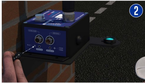
Caption 2: By Holding the magnet on the 'Hello!' label for more than 5s, the sensor wakes-up and transmits to the LoRawan network the data measurement followed by the system diagnostic ( battery status and network quality)
