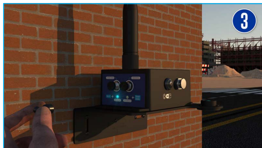
Figure 3 : The Activity LED blinks in blue, the sensor zeroing starts on both X and Y axis . When this process is done, the Activity led will blink again in blue color and transmits a data measurement to the Lorawan® network. If the sensor zeroing process is not done correctly [ the device is moving] the Activity Led will blink in Red color.
