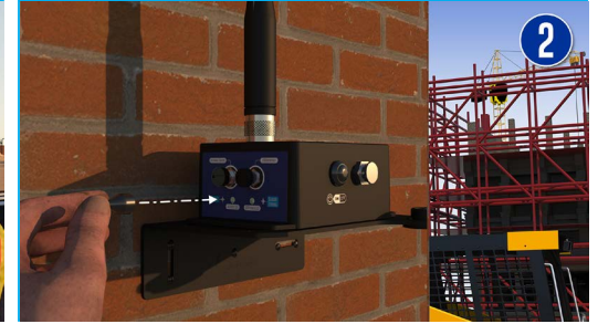
Figure 2 : By Holding the magnet on the 'Hello!' label for more than 10s, the sensor wakes-up and transmits to the Lorawan network the data measurement followed by the system diagnostic [ battery status and network quality].
