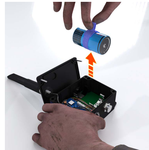
Figure 3 : Please do not use screwdrivers or other tools to remove the battery, as this may damage the circuit board.
