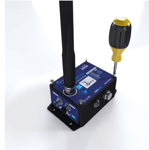
Figure 1 : Unscrew the 4 screws from the lid
