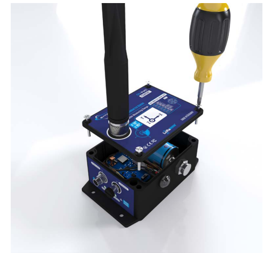
Figure 4 : Carefully replace the new Battery Type D-Type (only Lithium Thionyl-Chloride), then make sure that the case is securely closed.
