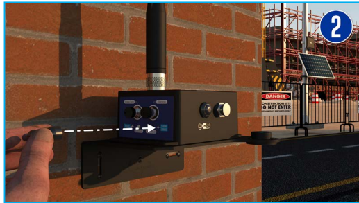
Figure 2 : To enable the sensor zeroing function, hold the magnet on 'Sensor Zeroing" Label for more than 10s.
