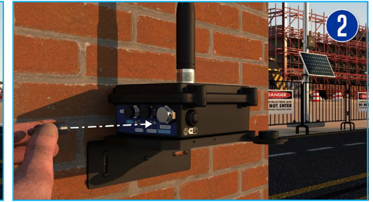
Figure 2 : To enable the sensor zeroing function, hold the magnet on 'Sensor Zeroing" Label for more than 10s.
