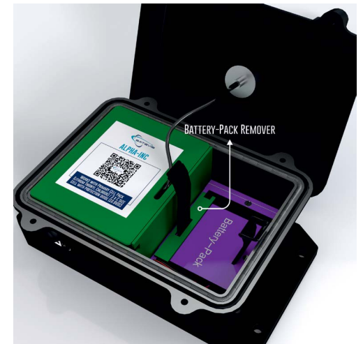
Figure 4 : You will find the "Battery-Remover" under the battery pack.
