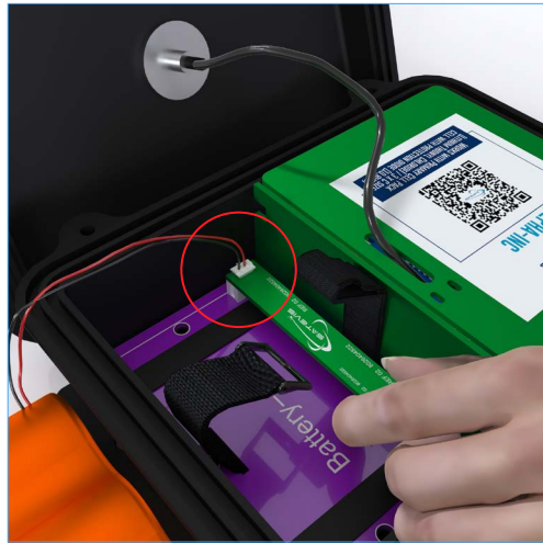
Figure 6 : Make sure the "battery-Remover" groove surrounds the connector.
