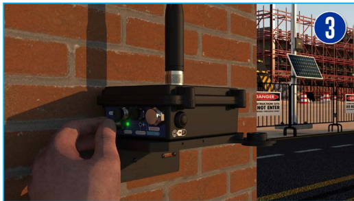
Figure 3 : The Activity Led blinks in green color , confirming that a data measurement is transmitted to the Lorawan network.
