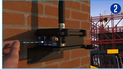
Figure 2 : By Holding the magnet on the 'Hello!' label for more than 10s, the sensor wakes-up and transmits to the Lorawan network the data measurement followed by the system diagnostic [ battery status and network quality].
