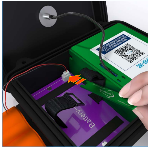
Figure 5: direct the "Battery-Pack Remover" towards the JST connector.
