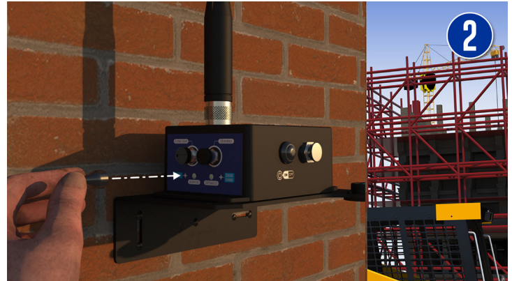
Caption2: By Holding the magnet on the ‘Hello!’ label for more than 10s, the sensor wakes-up and transmits to the Lorawan network the data measurement followed by the system diagnostic ( battery status and network quality).
