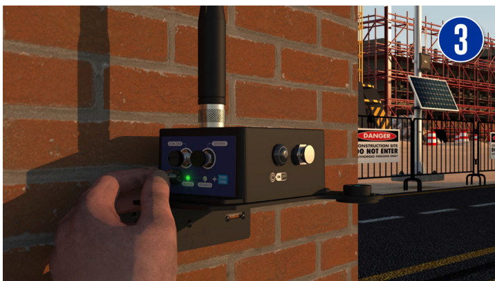
Caption3: The Activity Led blinks in green color , confirming that a data measurement is transmitted to the Lorawan network.
