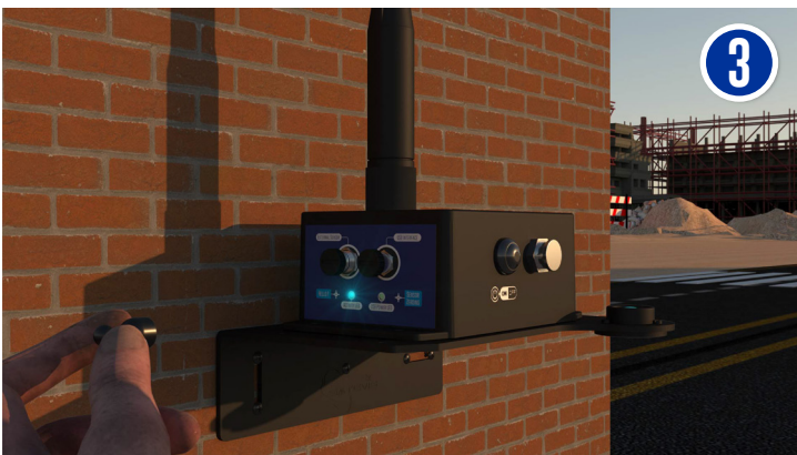
Caption3: The Activity LED blinks in blue , the sensor zeroing starts on both X and Y axis . When this process is done, the Activity led will blink again in blue color and transmits a data measurement to the Lo-rawan® network. If the sensor zeroing process is not done correctly ( the device is moving) the Activity Led will blink in Red color.
