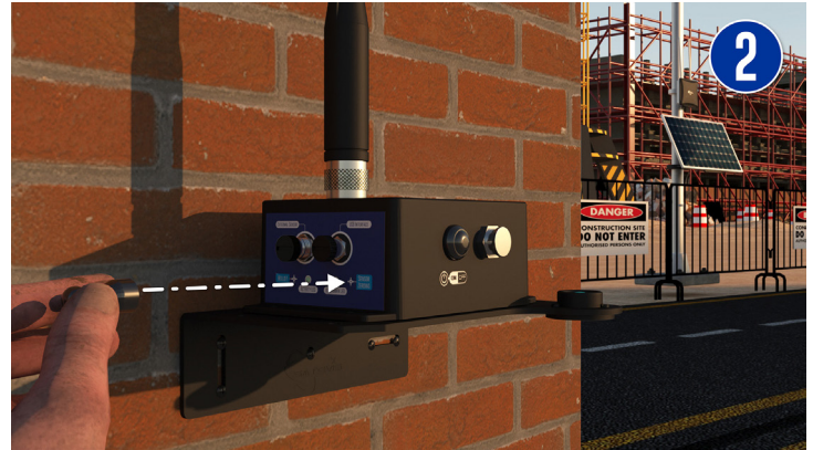
Caption2: To enable the sensor zeroing function, hold the magnet on 'Sensor Zeroing' Label for more than 10s.
